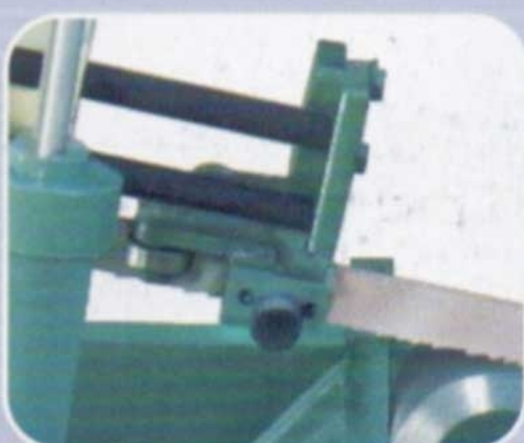
Improved blade guide mechanism (Carbide & bearings for HS models)
