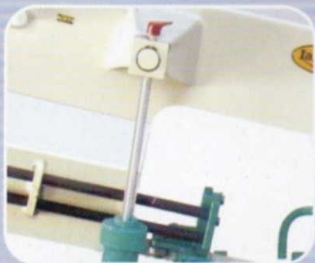
Adjustable cutting feed control valve
